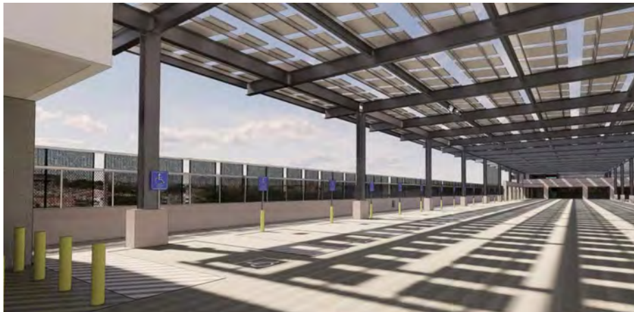
Figure 10 – Example, Canopy Mounted PV System
