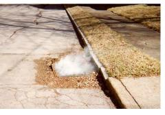
Smoke Testing reveals a storm drain improperly plumbed to the sanitary sewer collection system.
