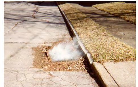
Smoke Testing reveals a storm drain improperly plumbed to the sanitary sewer collection system.
