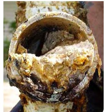
*Disposing of fats, oil and grease down the drain can quickly lead to clogs like this! Do your part to keep it out of the sewers.*
